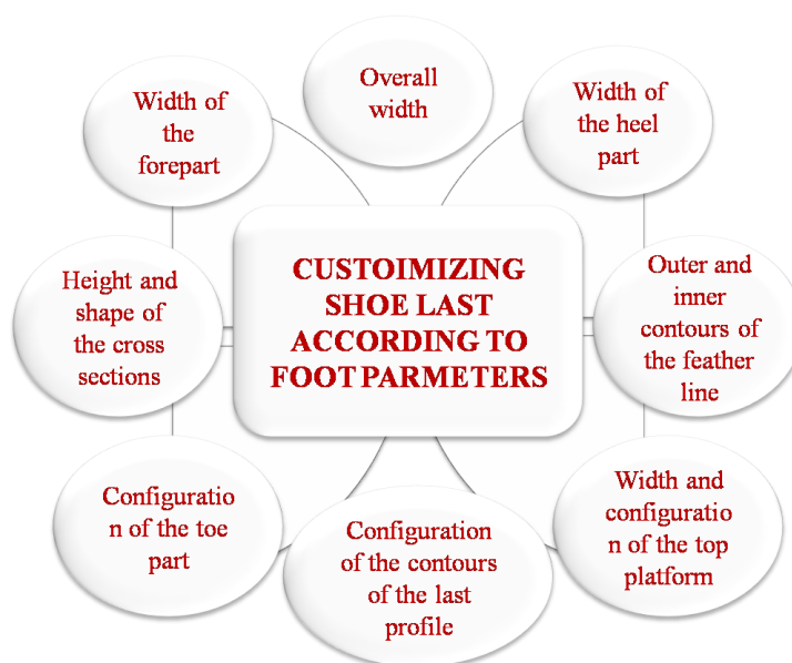
Figure 5: the main operations of the shoe last modeling in the 3dCAD using reverse engineering.
