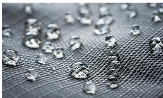
Figure 16 Lotus effect on textile material [11].
